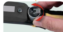
扭力調整旋鈕 Knob type torque adjustment
